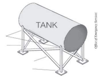
Figure 49–Bracing tanks. Tank supports should be cross-braced as well as bolted to the floor.
