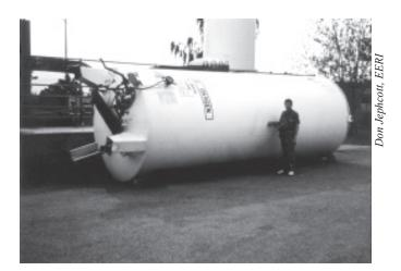
**Figure 46** - The support pedestal system of this oxygen tank at Olive View Medical Center was damaged after the 1994 Northridge earthquake, leaving the tank leaning. The tank is shown after it was removed to allow for installation of a replacement unit.
