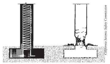
**Figure 24** - The addition of more confining steel (c) keeps the vertical reinforcing bars from buckling and the concrete from shifting so that the building continues to be fully supported (d) even it if is damaged in an earthquake.
