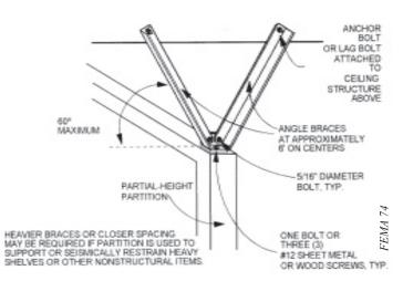
**Figure 61** - Adding braces to the top of free-standing partitions can prevent them from toppling.
