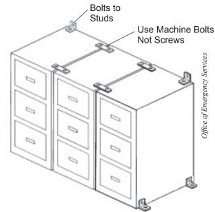
**Figure 45–Bolting file cabinets.** Bookcases and file cabinets should be bolted to the wall and to each other to keep them from falling. File drawers should have latches so they can't open in earthquakes.
