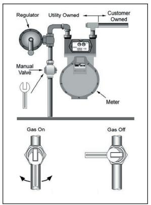
Figure 64—Manual Shutoff Valve Location
