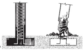
**Figure 21 –Lack of Reinforcing steel.** If the confining reinforcing steel in a column is too widely spaced (a), it will not be able to keep the vertical reinforcing bars and the concrete in place when it is shaken by an earthquake (b).
