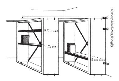
**Figure 43–Securing shelves and furniture.** Attach rows of shelving and other tall pieces of furniture to the wall and to each other for support; tilt the shelves or install shelf parapets or other restraints to keep objects from falling off shelves.
